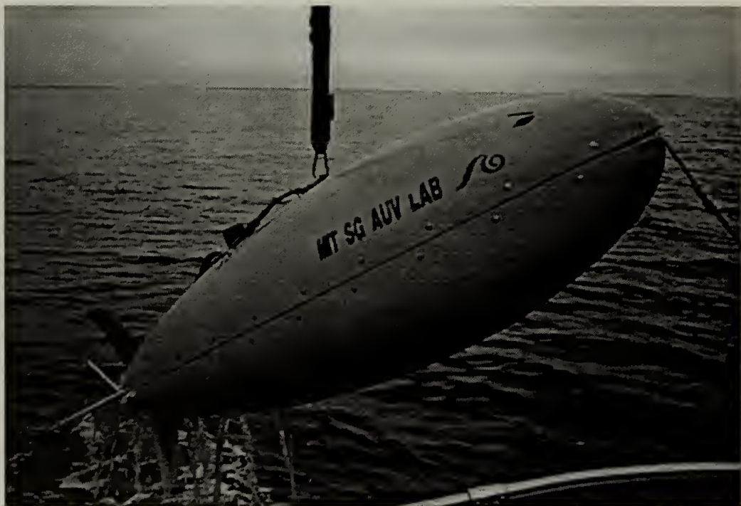
Figure 2: The Odyssey II AUV [MIT Home Page 96].
